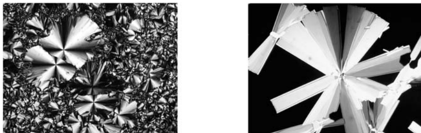
FIGURE 1 Typical structure found in the liquid crystalline phase of nitrogen centered achiral amide disk 3a (left) and crystals of chiral amide disk 3b (right). (See Color Plates XVII & XVIII).
